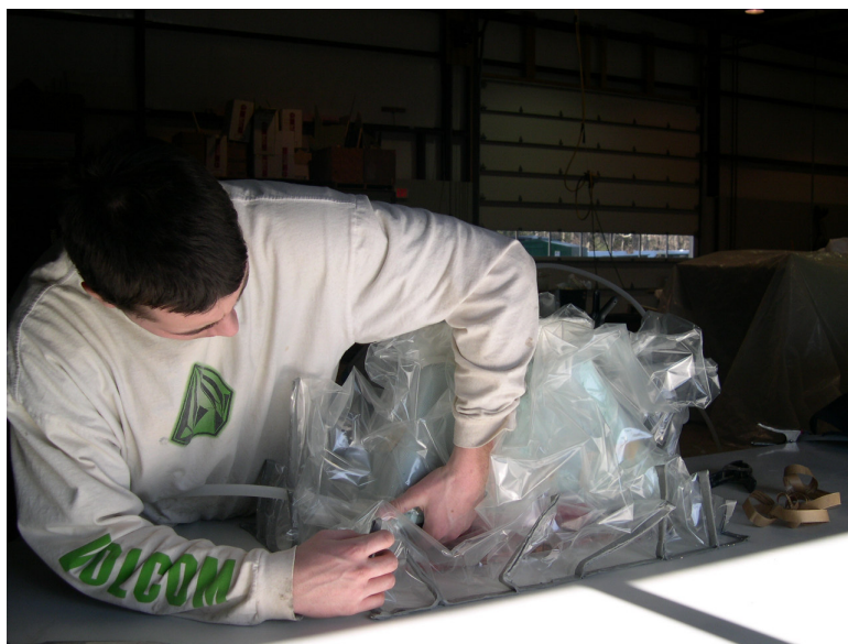
CCTI employee Joe Alexander infusing a composite railroad connector.
