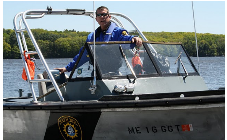
Specifications: Length: 21'; Engine: 200 HP Volvo Diesel; Hull: Aluminum; Full Capacity: 100 gal. diesel
