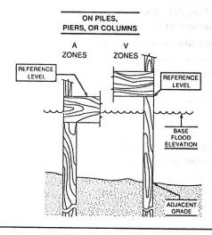
The diagrams above illustrate the points at which the elevations should be measured in A Zones and V Zones.
